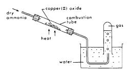
Ammonia was passed over the red-hot copper(II) oxide. As soon as the air was displaced, the test tube was put in position. The gas collected was
